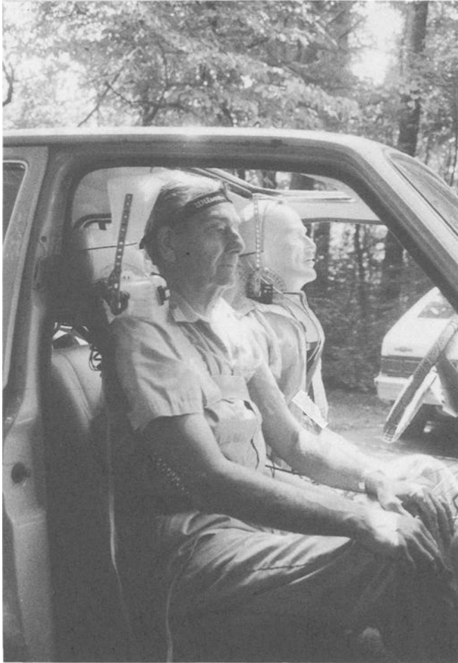
FIG. 6—Side by side volunteer and manikin instrumentation.
